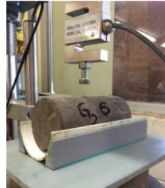
Figure 2 Needle penetration resistance test system
