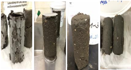
Figure 6 Soil-cement samples exposed to 1000% SW (from left to right: 42, 58, 118 and 208 days)
