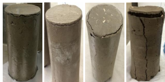
Figure 4 Soil-cement samples exposed to 200% SW (from left to right: 42, 58, 118 and 208 days)
